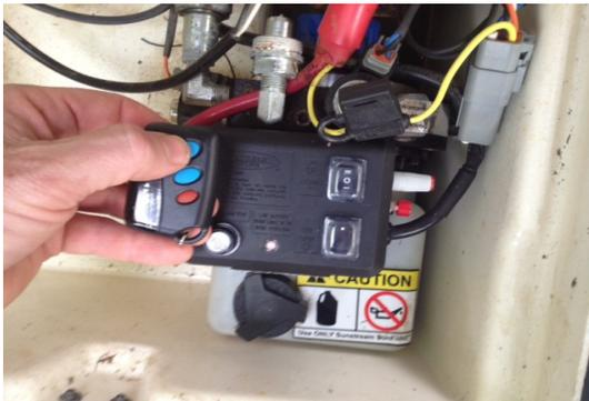
Repeat for each remote that you want to pair to that base unit. If you have a handheld that controls more than one lift at the same time, then press and hold the red bottom on the side of the base unit for 15 sec. And it will clear all the handhelds. After clearing all handhelds for that lift, reprogram the correct handheld to that lift using the above procedure in Step #1.
